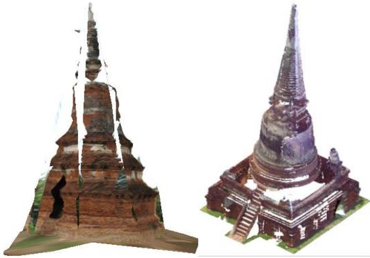
Fig. 5 – examples of 3D models: left – Wat Lang Kha Khaow from the photogrammetry method; Right – small chedhi from the LIDAR method
